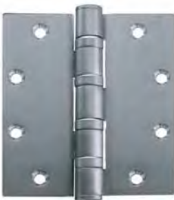
SY-FBB168-4-1/2X4-26D ANSI A8111 - Steel For heavy doors or doors where high frequency is expected, such as entrance doors to office buildings, stores, public buildings and corridor entrance doors to offices All hinges have template screw hole location for use on either wood or hollow metal doors and frames
